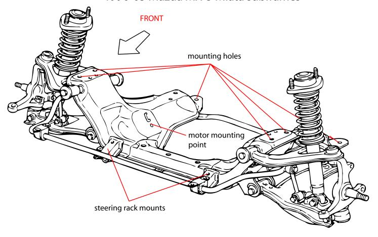
Shock upper mounting points are not crucial to suspension geometry front or rear.
